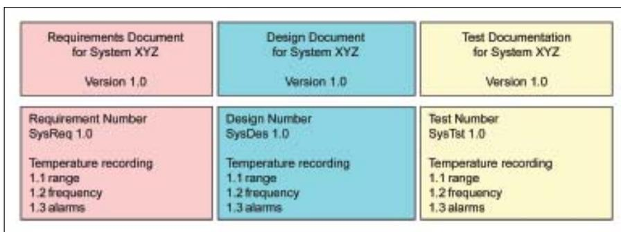
Figure 2. Example of embedded traceability for simple systems.
