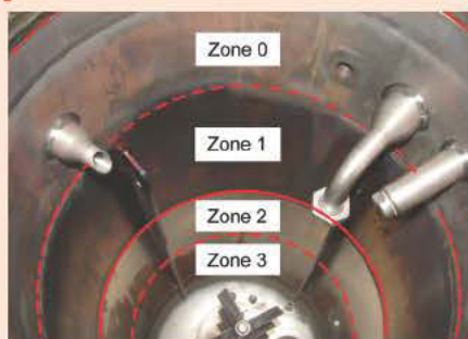
Figure 16 Classification of the interior space of the test tank into zones with different rouge formation
