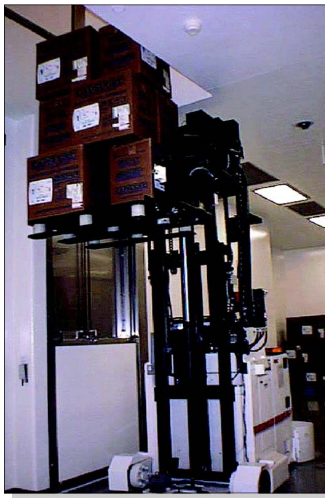
Figure 6. Turrent SGV moves pallets of raw material.
