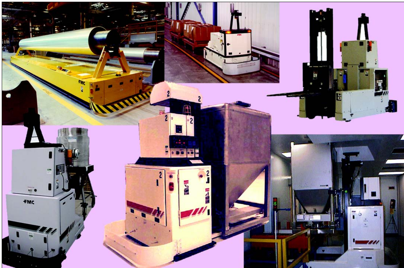
Figure 2. Front - three fork style SGVs carrying totes, rear-large load, tugger, and reach SGVs.
