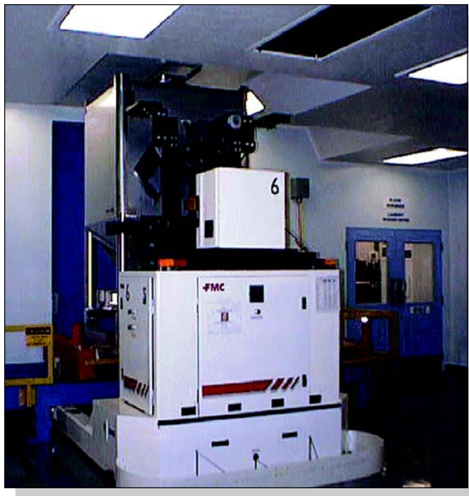
Figure 5. Fork SGV places stainless steel bin on receiving stand.
