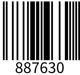
FIGURE 1: A ONE-DIMENSIONAL BAR CODE.
